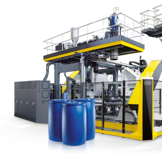
thicknesses, which are not possible with other electric clamping drives of large blow molding systems. This ensures quick adaptation to their specific requirements. The molds themselves can be easily and quickly exchanged from the side by means of quick change plates, and centering devices immediately returning the mold to its original position. As the design of the clamping drive is unique in industrial blow molding machine applications, it is a patent pending feature.
