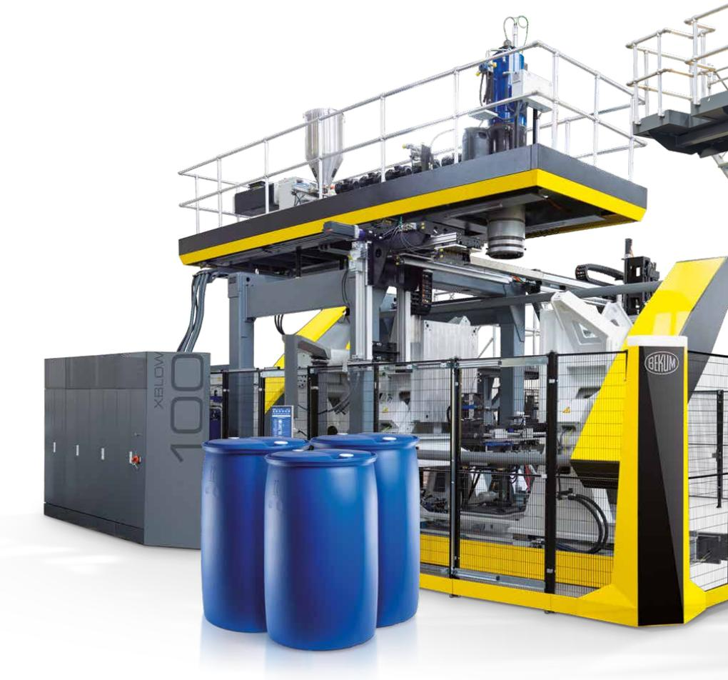
thicknesses, which are not possible with other electric clamping drives of large blow molding systems. This ensures quick adaptation to their specific requirements. The molds themselves can be easily and quickly exchanged from the side by means of quick change plates, and centering devices immediately returning the mold to its original position. As the design of the clamping drive is unique in industrial blow molding machine applications, it is a patent pending feature.
